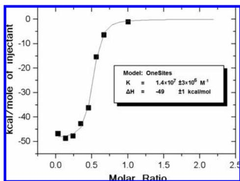
**Figure 4.** Measurement of the dissociation constant of the complex between TNT and the peptide TNT-BP determined from isothermal titration calorimetry. Data points (values for the integrated heat change during each injection, normalized per mole of TNT) are represented by filled squares. A one-site model was used to fit the data. The solid red line is the calculated curve using the best-fit parameters.
