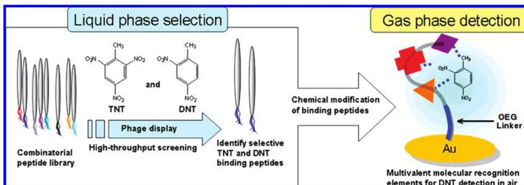
**Figure 1.** Schematic diagram showing our biomimetic approach to develop selective coatings for gas-phase explosive molecules. Identified molecular recognition elements from the directed evolution process of phage display are used for their multivalent recognition of explosive targets in liquid-phase screening. Through chemical modification, the peptide receptors are linked with oligo(ethylene glycol) and immobilized as coatings capable of binding explosive targets in air.
