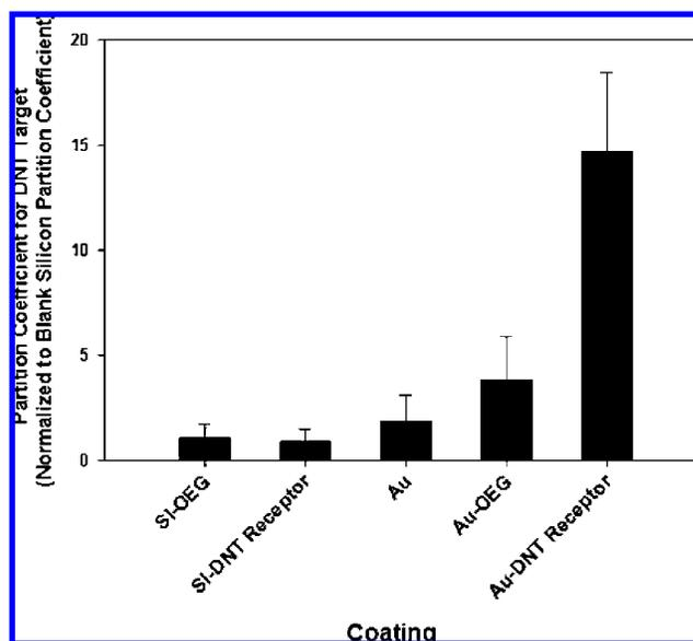
**Figure 5.** Gas-phase screening for partition coefficients of various coatings on Si exposed to DNT gas. The values are normalized to the DNT gas partition coefficient of blank Si substrates to observe the contribution attributed solely to the coating layer. Partition coefficients are calculated as the ratio of the concentration of analyte bound to the coating (identified through thermal desorption GC-MS) to the concentration of analyte in the exposed gas headspace.
