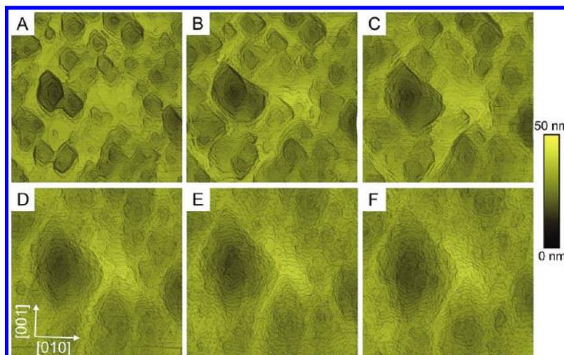
**Figure 4.** Step roughening under  $10\ \mu\text{M}$  NaF concentration (size:  $1.4 \times 1.4\ \mu\text{m}$ , sequential AFM images with time interval 40 min). Between image frame (C) and (D), the dissolving solution condition is changed from pH = 6.0, no salt concentration, into pH = 6.0,  $10\ \mu\text{M}$  NaF concentration. The right color bar represents relative vertical profile.
