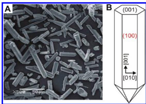
**Figure 1.** Hydroxyapatite structures. (A) An SEM image of single crystalline HAP. (B) A model of an elongated hexagonal rod-shaped HAP crystal. The specific crystallographic directions and facets are indicated.
