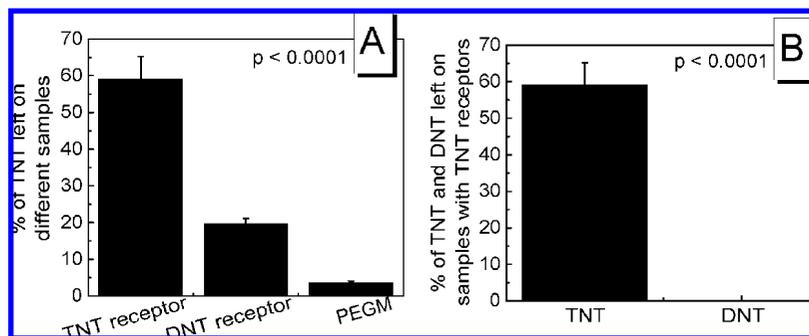
**Figure 7.** GC/MS measurements of (A) the amount of TNT remaining on samples containing TNT receptor, DNT receptor, and just PEGM after overnight washing in water and (B) the amount of TNT and DNT remaining on samples containing the receptor specific for TNT, after overnight washing in water. Amounts are given in pmoles, calculated as described in the “Material and Methods” section. Details about  $p$  values calculated according to Student’s  $t$  test are reported in the text.
