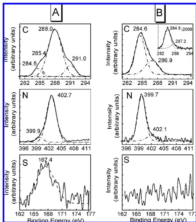
**Figure 3.** XPS spectra of C 1s (first row), N 1s (second row) and S 2p (third row) peaks of TNT receptor deposited on a bare Au slide before (column A) and after (column B) washing in water overnight. Experimental spectra are plotted in solid line, fitted spectra in dashed line, and fits for each peak component in dash-dotted line. The inset in the C peak, column B, represents the C 1s spectrum recorded on a bare Au substrate.
