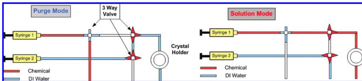
**Figure 2.** Schematics showing the two modes of operation of the QCM setup.
