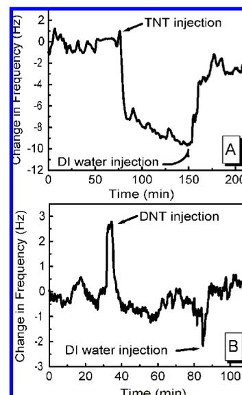
**Figure 8.** Change in QCM resonance frequency measured on a crystal coated with PEGM/TNT receptor, after exposure of a solution containing TNT (A) and DNT (B), respectively.
