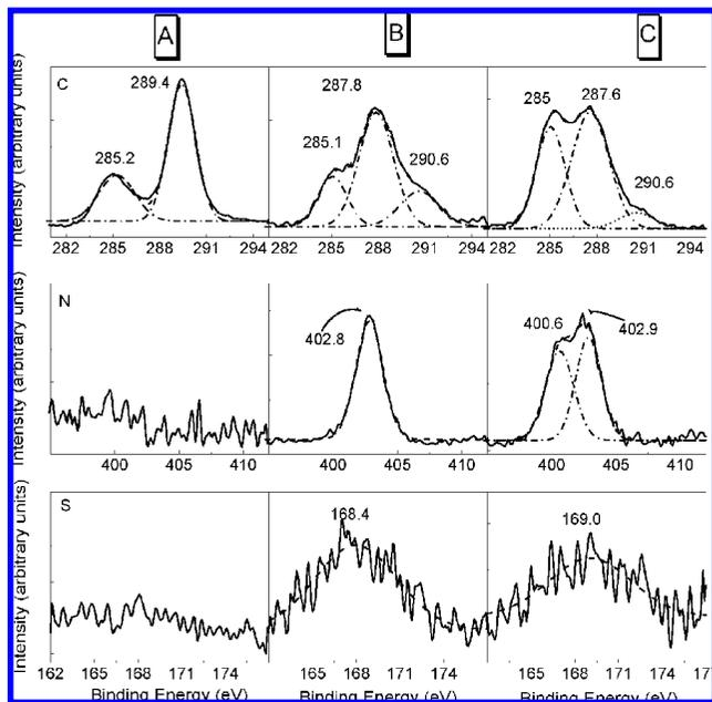
**Figure 4.** XPS spectra of C 1s (first row), N 1s (second row), and S 2p (third row) peaks of PEGM deposited on Au (sample “PEGM/Au”) (column A), and TNT receptor bound to PEGM on Au (sample “TNTrec/PEGM/Au”) before (column B), and after (column C) washing in water overnight. Experimental spectra are plotted in solid line, fitted spectra in dashed line, and fits for each peak component in dash-dotted line.
