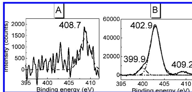
**Figure 5.** XPS spectra of N 1s region for samples prepared by deposition of 660 nmol of TNT on (A) PEGM/Au and (B) PEGM with TNT receptor. Experimental spectra are plotted in solid line, fitted spectra in dashed line, and fits for each peak component in dash-dotted line.
